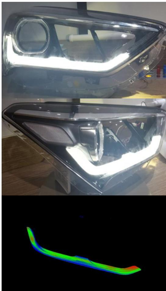
Prior to applying the back cover, there was not enough light like the yellow area above, and there was a dark area. Before applying back cover optics, camera Check the measurement results, you can see that there are many red areas showing dark are-
