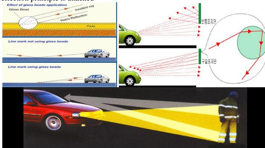
**Fig.7** Application of Retro-Reflection Principle
