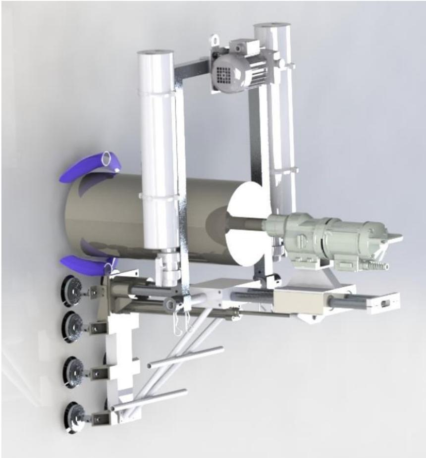
Fig. 4. Model of vacuum-fixed drill
